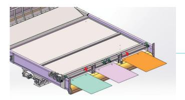
That can adjust the shooting tunnel is internal working width according to
