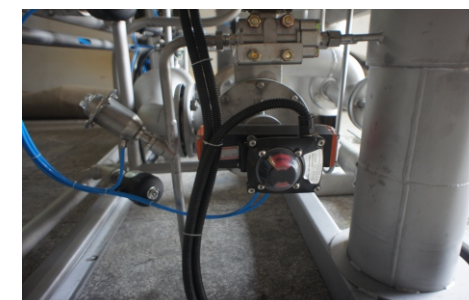
风动换向装置 Pneumatic Flow Reverse Device
