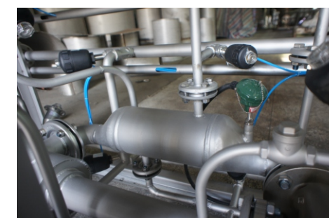
独立热交换器 Independent Heat Exchanger for precise temp control
