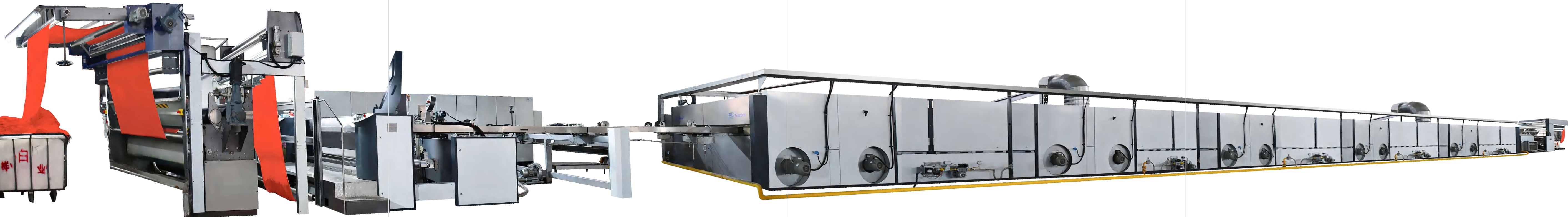
For knits: 1 correction roller and 1 scroll roller 针织物两用：1根导布辊+1根螺旋扩幅辊
